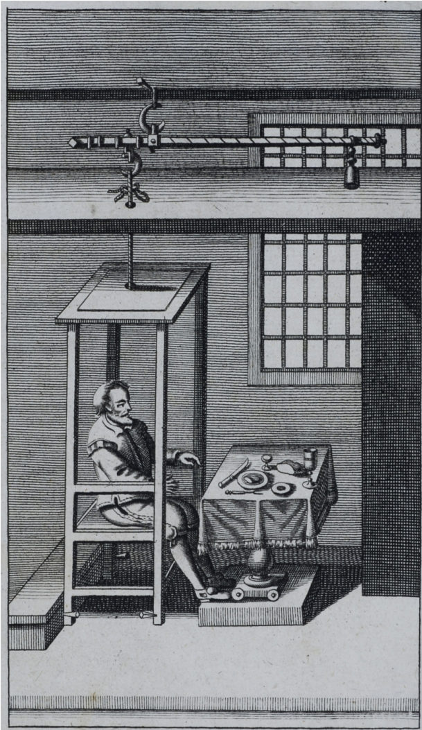
Illustration from a 1723 English edition of Italian physician Santorio Santorio's Medicina statica , showing the apparatus he built to weigh himself and what he consumed and excreted.
